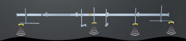
As a combination, **MOBA-matic** and the sensor solution **Big Sonic-Ski** with up to 4 ultrasonic sensors are absolutely unbeatable! Thanks to a span of up to 13 m, even long ground waves are completely levelled out and eliminated. This unique feature ensures an exceptionally flat surface and makes the system not only the most precise technology on the market, but also an absolutely groundbreaking solution. Welcome to road construction of the future!
